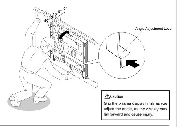
8. Fasten the Angle Adjustment Lever.
